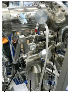
2D detector | SCIENTA R2002 Rice Univ. type Mott detector(30-35kV)
