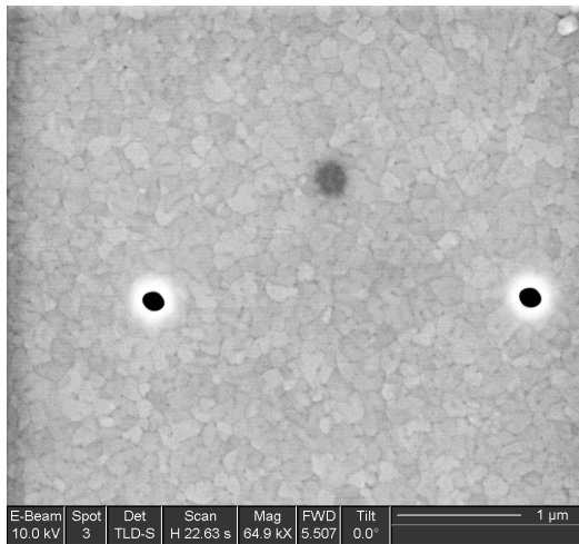
sample#2 \Phi=170\text{nm} , d=3\mu\text{m}
