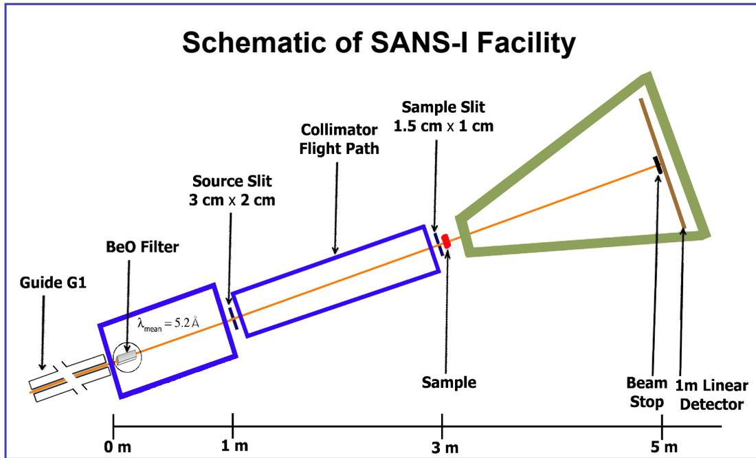
Fixed Geometry Instrument covers a Q range  $0.015 - 0.35 \text{ \AA}^{-1}$
