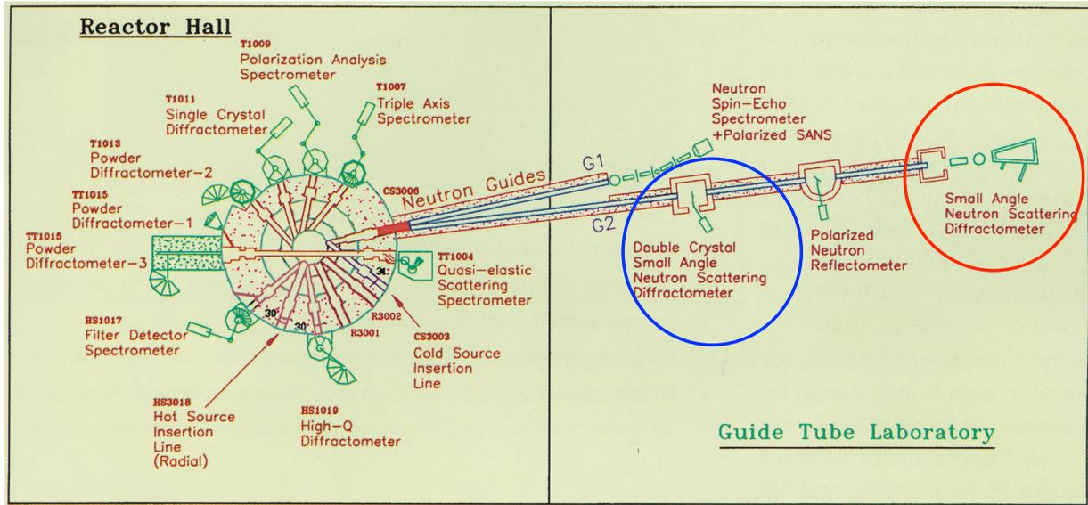
**Layout of the NBR facility at Dhruva Reactor, BARC, INDIA**
