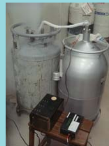
Fig.5 Test setup of Pump A Right: storage tank (alloyed Al.) Left: target tank (stainless)
