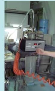
Fig.6 Test setup of Pump B storage : glass insulated dewar tank
