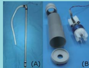
Fig.3 Pump A (A)with transfer tube (B)overhauled
