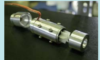
Fig.4 Pump B (overhauled)
